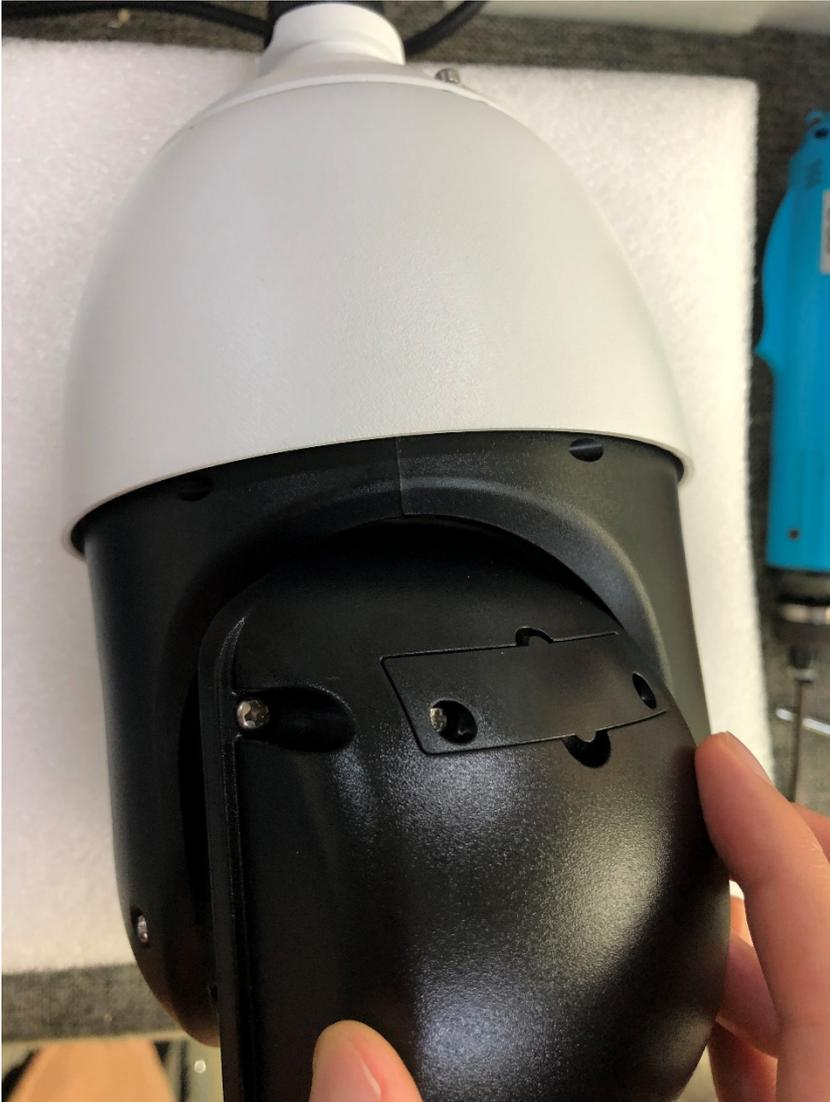
Step 3. Locate the TF Card Slot, and insert the TF Card.
