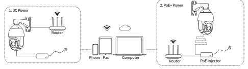
The camera can also be connected to a PoE injector/switch which would let the network cable supply both power and data connection.
